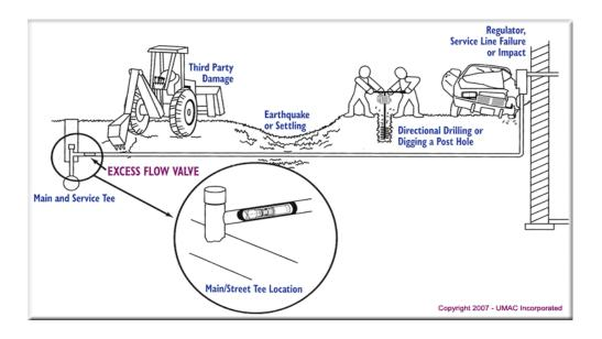
Residential and small commercial customers whose total gas appliance load is no greater than 1,000 cubic feet per hour (approximately 1,000,000 BTU per hour) may request EMU to install an EFV in their service line if one does not already exist. Other technical requirements must also be evaluated to determine whether an EFV will properly function on any given gas service line.
