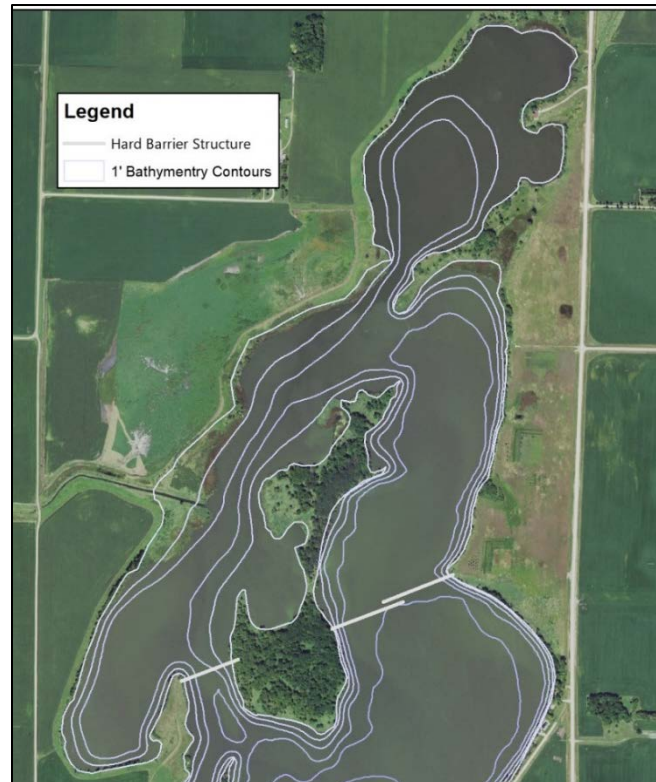
Figure 29 – Hard Barrier Structure
